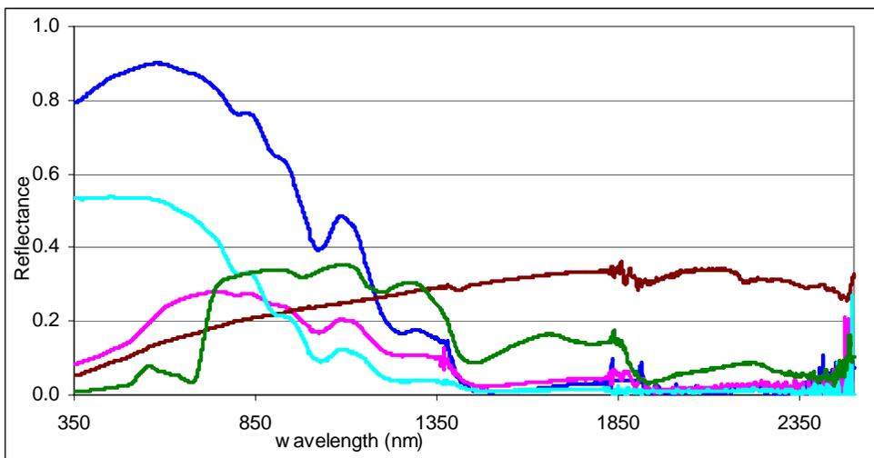
**Fig. 1** Spectral reflectance of snow, ice, contaminated snow, vegetation, and soil. These observations were taken using spectral radiometer near Manali, Himachal Pradesh. Please note changes in reflectance as snow changes into ice and as snow and ice is covered by rock debris.
